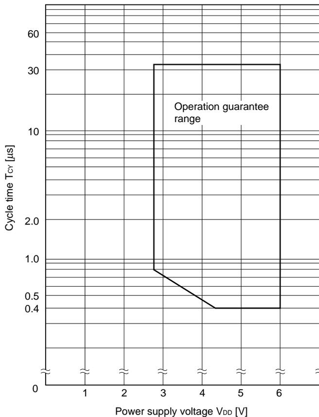
(2) Serial interface (T<sub>A</sub> = -40 to +85 °C, V<sub>DD</sub> = 2.7 to 6.0 V)
