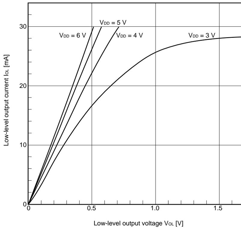
$I_{OL}$  vs.  $V_{OL}$  (Port 7)
