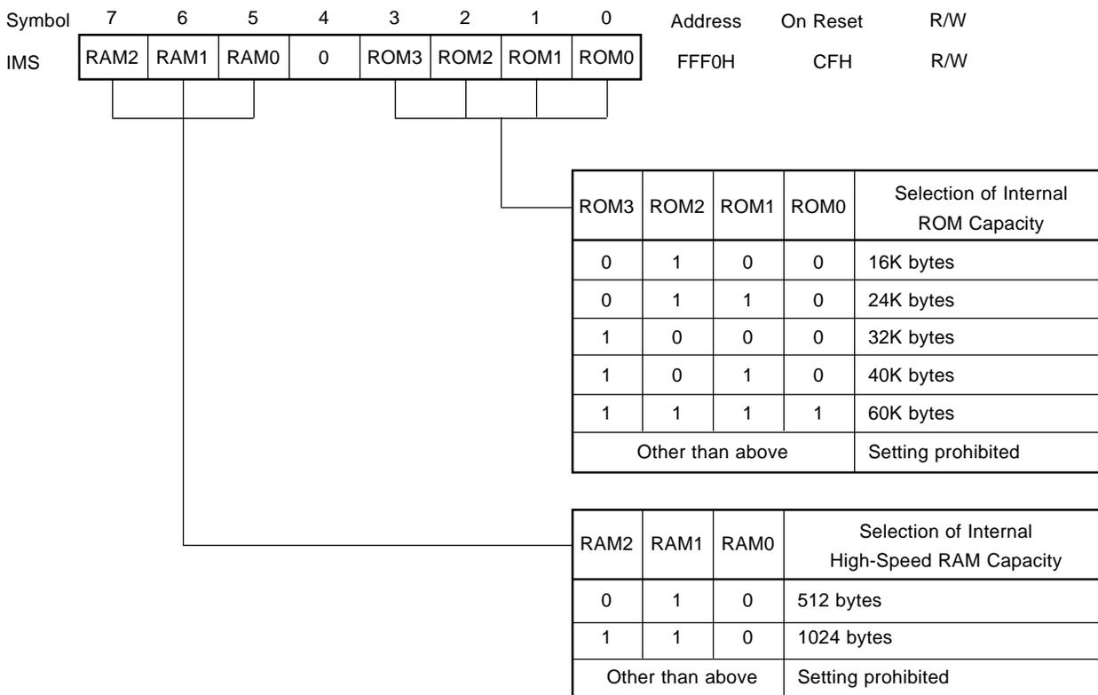
Table 3-1 shows the setting values of IMS which makes the memory mapping the same as that of the various mask ROM model.
