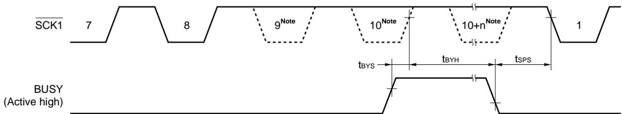
**Note** Though it does not become low level actually, have described as it does due to the timing rule.
