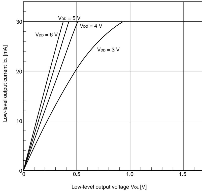
**I<sub>OL</sub> vs. V<sub>OL</sub> (Ports 0, 2, 3)**
