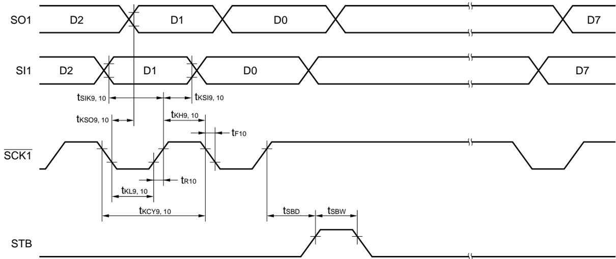
3-wire serial I/O mode with automatic transmit/receive function (Busy processing):
