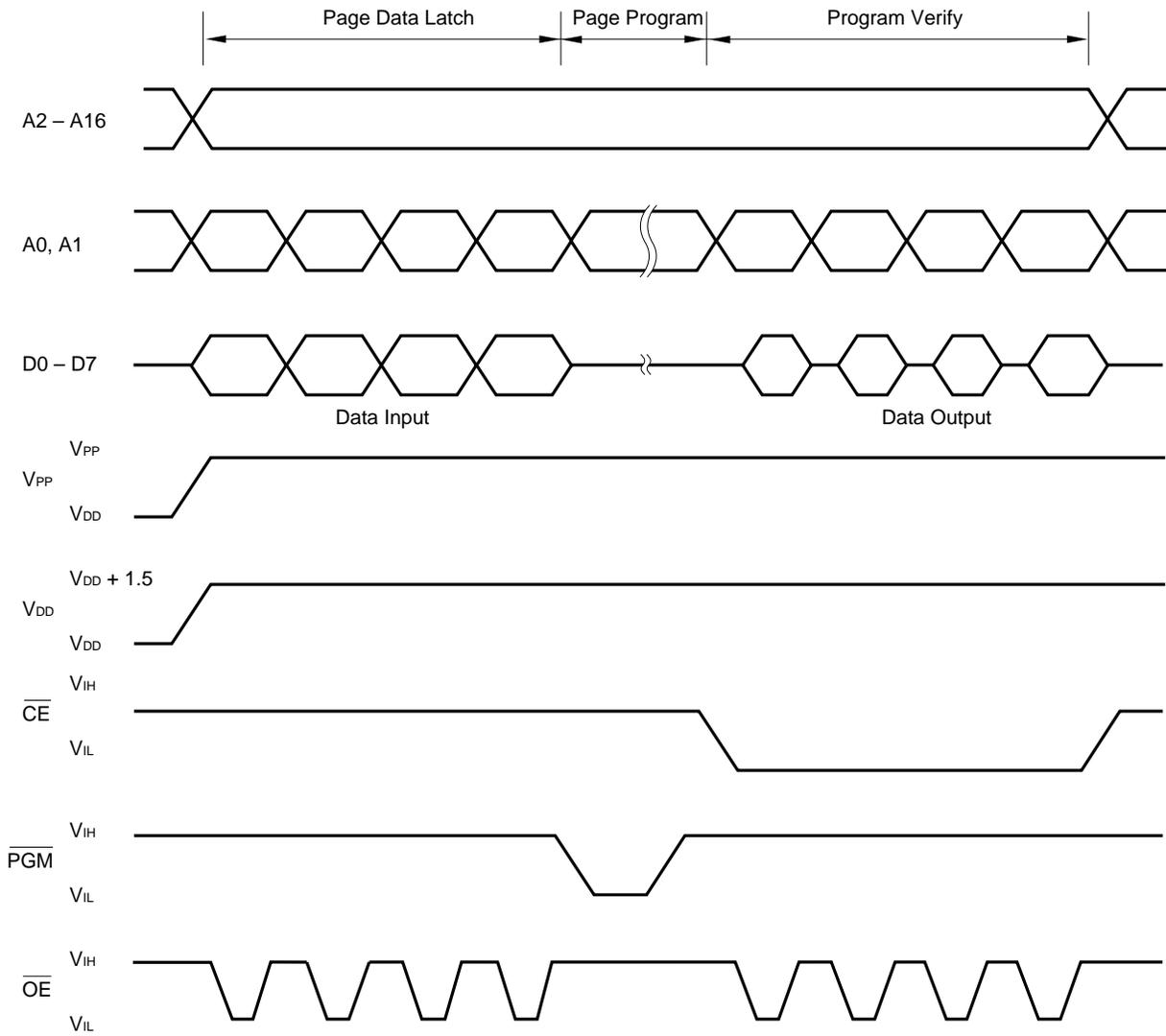
Figure 5-3. Byte Program Mode Flow Chart
