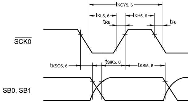
3-wire serial I/O mode with automatic transmit/receive function:
