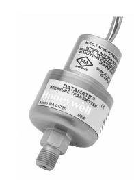
The Datamate is a two-wire pressure transmitter which is compatible with data loggers and instrumentation used in processing environments. Its 4 mA to 20 mA output is ideal for remote monitoring of both primary and secondary process variables.
