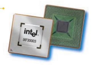
(OCOH) allow remote management of the optical network. Manufactured in a low-power 0.18µ CMOS technology, the IXF30003 can be controlled using an 8-bit processor interface, which allow high event-driven communication and reduced processor load.
